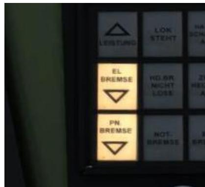
Every time the loco has come to a complete stop a light indicating “Lok steht” (loco stationary) will come on.
