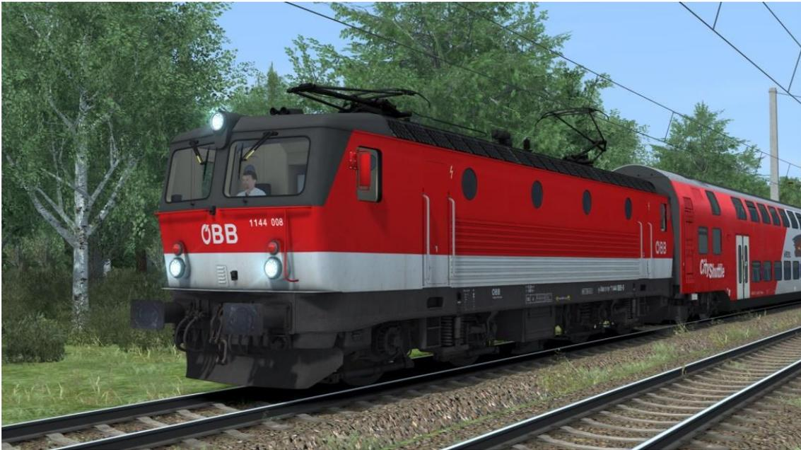
1144 with small/ low Fans (original version of this loco) – old and faded
