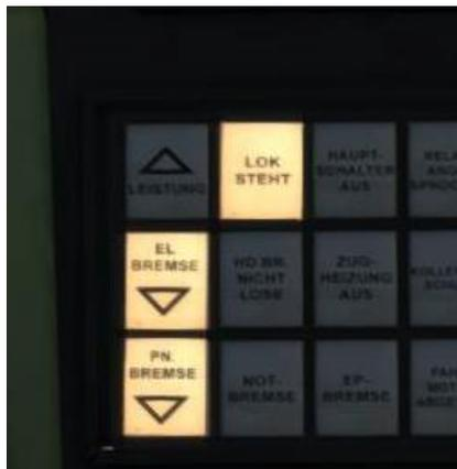
It is important to note that whilst the “PN Bremse” light is on, the loco will not be able to move forward. Also when releasing the brakes to accelerate again you need to first move the lever to the neutral position and wait for the “EL Bremse” lights to go out before moving it into the “Fahren” notch again. Once you have done that, again wait until the “Leistung” light comes on and you can add power.
