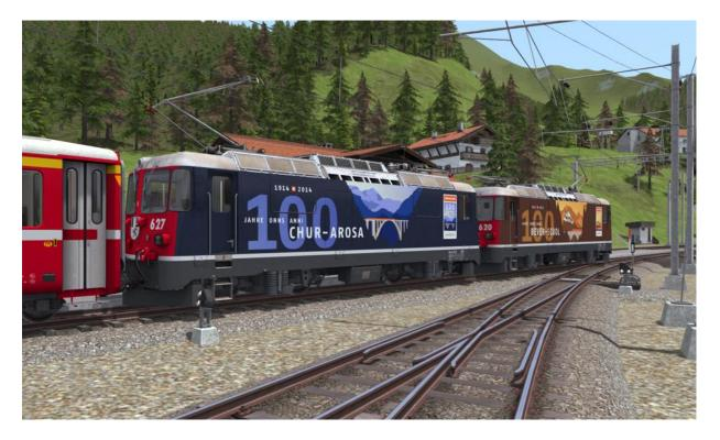
When operating Ge 4/4 II locomotives in pairs the automatic multiple working mode will be activated. This mode enables the front pantograph on the leading locomotive for use instead of the rear pantograph. Once uncoupled the locomotives will return to standard operation.
