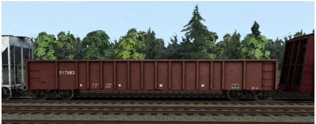
A open gondola can be used for loose bulk goods as well as materials for track maintenance.
