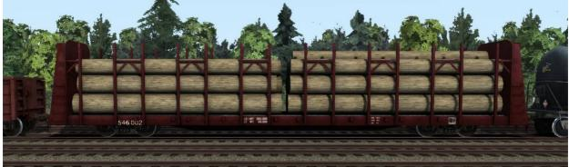
A Bulk Head Flat can be used to transport long bulky commodities. A load of logs and pipes are included.
