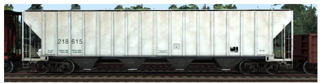
A covered hopper can be used to move bulk agricultural products as well as other bulk products
