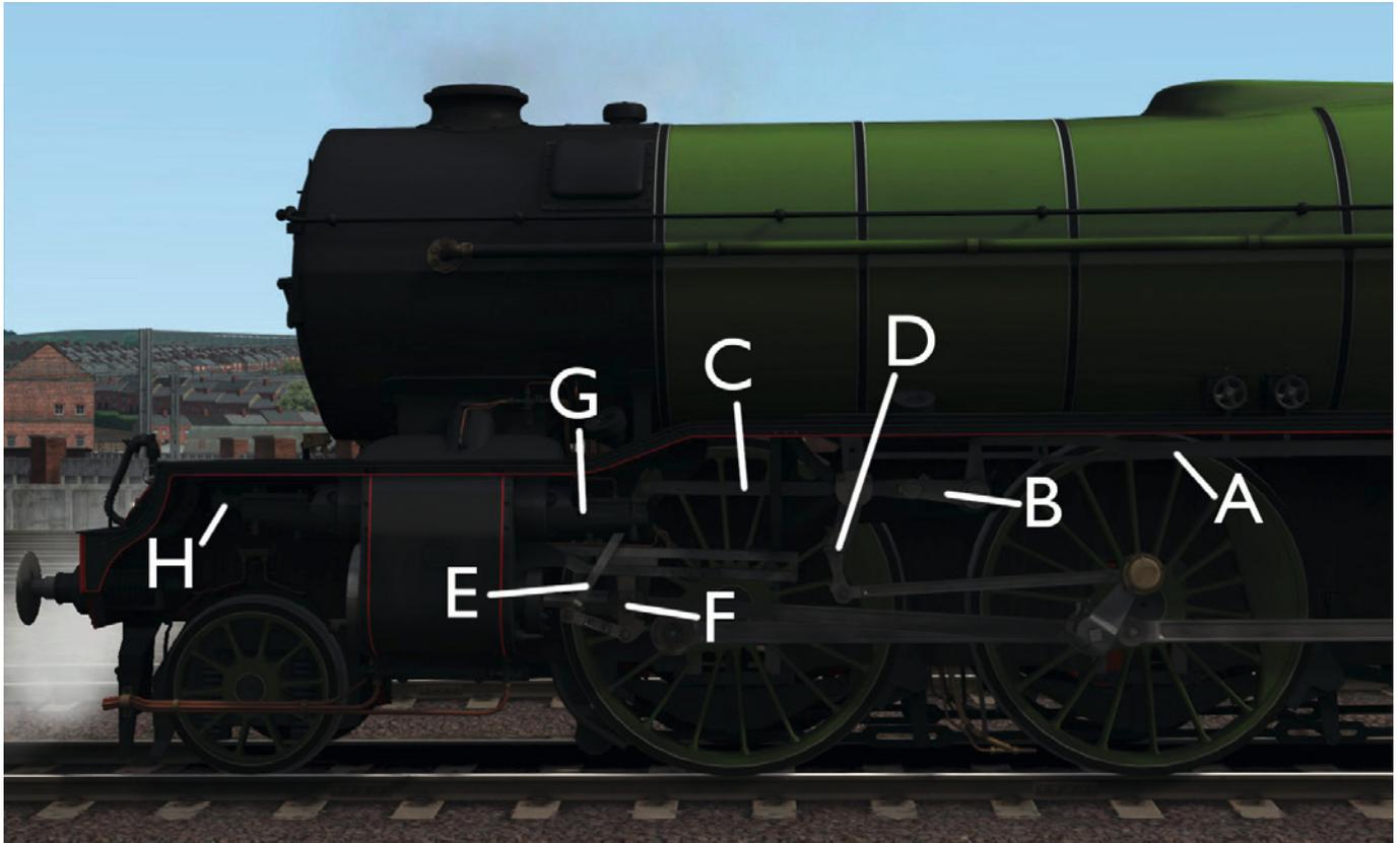
The valve gear is designed to control the ‘cut-off’, the point at which the piston valves prevent the further admission of steam into the cylinders. With the V2 and its Walschaerts valve gear, this is done by using the reverser in the cab to rotate a screw inside the reverser stand, that in turn draws a long rod (A) backwards and forwards between the cab and along the top of the running plate to the lifting arm (B).
