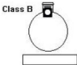
**Class B** – stopping passenger, rail motor or a breakdown train returning from a job
