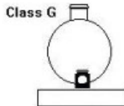
**Class G** – light engine or engine with one or two brake vans attached
