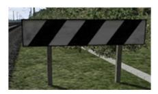
Ra 10 "Yard limit sign" Shunting is not possible from the signal onwards.
