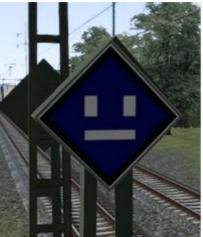
El 2 "Switch-on" of the main switch of the Elocomotive again. Only function together with virtual Railroads "Expert Line" locos.
