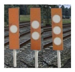
Zs 1 "Substitute signal" Signal indicating "Stop" or which is disrupted should be ignored without written order. (A flashing white light)
