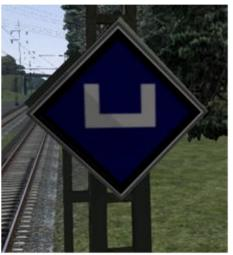
El 3 Expect the signal "Pantographs down". In breaking distance follows EL4, where pantographs have to be lowered.
