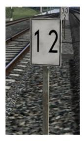
Ne 2 "Advance signal board" Marking of the location of a distant signal
