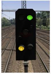
HI6a "Drive at 40 km / h then at 100 km / h"
