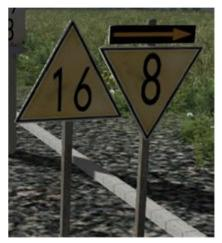
Lf 7 "Speed board" The speed indicated in the signal (number x 10) must not be exceeded from this signal onwards.
