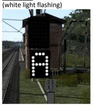
Zs 3 "Speedometer" The indicated (numbers x 10 in Km / h) speed not be exceeded in the turnover area from the signal onwards.
