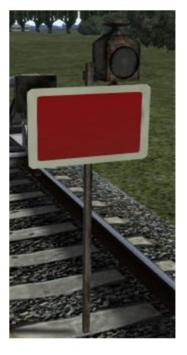
So 19 "Main signal board" A main signal can be expected.
