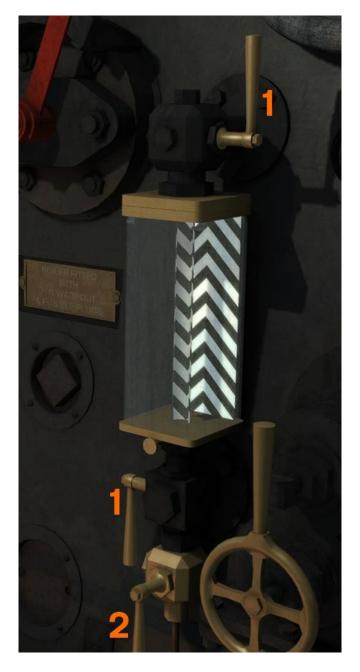
You can also perform blow down tests on the gauge glasses by doing the following:
