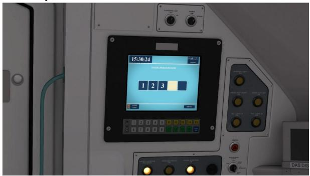
The 180 features a TMS system to the left of the Driver. This provides information to the Driver about the trainset. By default you will be greeted by a login screen for the system. Using the keypad entry below, enter a five digit number sequence to access the overview screen. If you are presented with a "Cab Not in Service" screen then you will need to ensure the Master Key is engaged.
