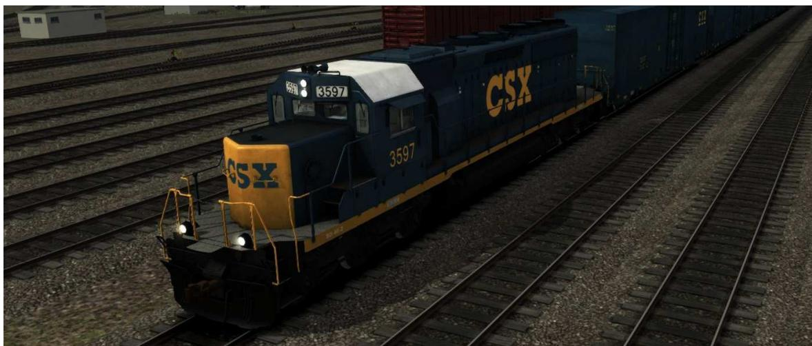
Introduced between 1972 and 1986, General Motors Electro-Motive Diesel (EMD) produced the SD40-2 as a 3,000 horsepower model as an upgrade from the SD40. Although not as powerful as some rival locomotives in the same Class, the SD40-2 features modular electronic control systems, making it significantly more reliable and economical than its competitors.
