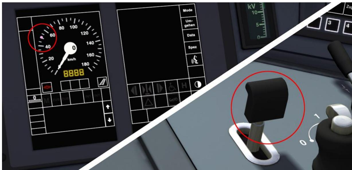
The RABe 523 is equipped with automatic speed control. The desired maximum speed for the line ahead should be selected using the V-Controller Lever and this will be indicated by the moving V-Controller Speed Indicator on the Speedometer. Speed selection can be made in 5 km/h increments from 5 to 160 km/h. Changes to the selected speed can also be made using the “Y” and “C” keys on the keyboard.
