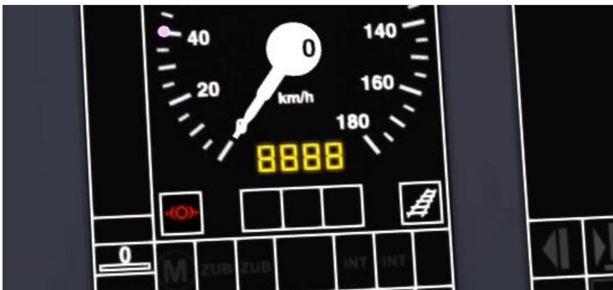
You are alerted by the Zub safety system when you pass a distant signal (Vorsignal) that is displaying a warning. The Zub display will show the target speed in km/h that you must achieve before reaching the next main signal where the target speed restriction will begin. If the distant signal is warning of a danger (stop) signal ahead then the target speed will be zero and the display will show "0".
