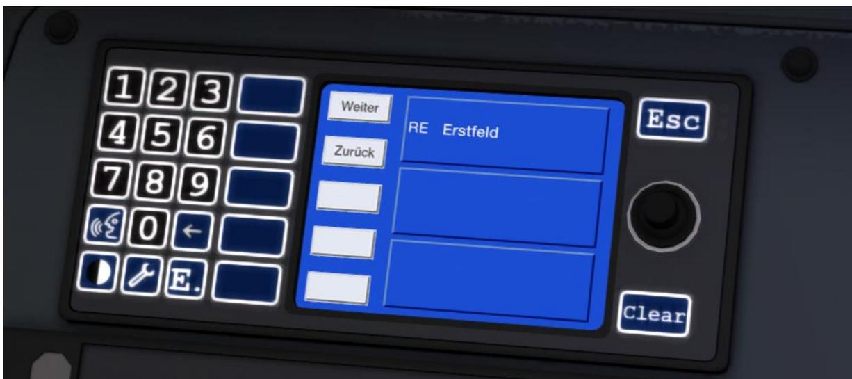
The display boards are controlled via this interface. There are 14 keys the driver can interact with to input a route.
