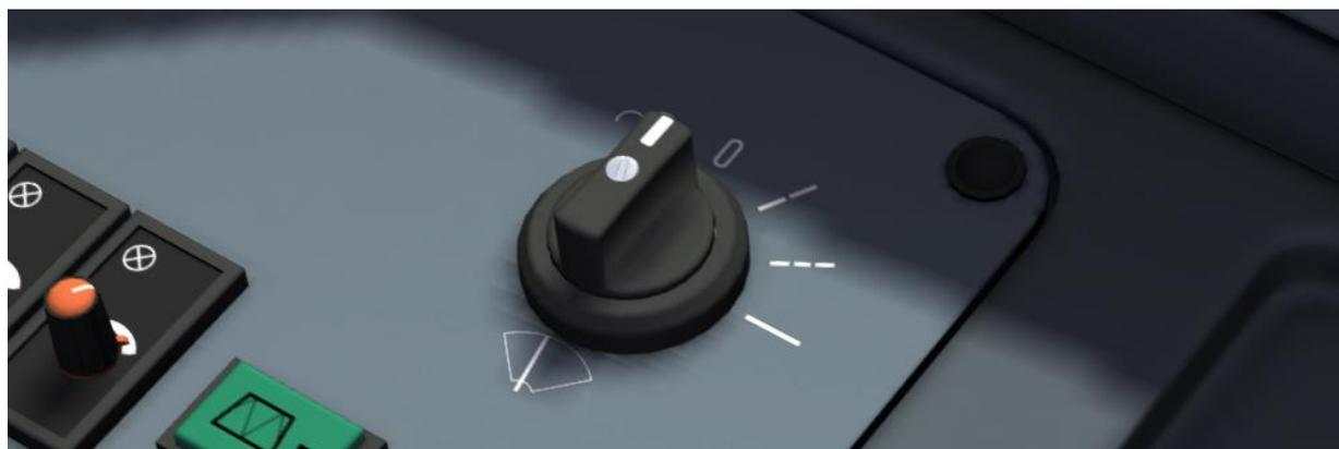
The windscreen wipers switch has four positions. Off, Intermittent, Slow and Fast. On the keyboard use key “V” to increase and both keys SHIFT and ”V” together to decrease the current setting.
