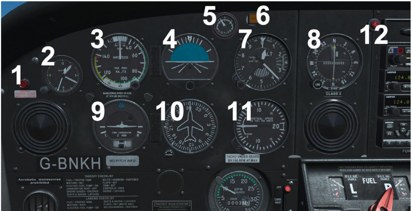
1. Engine starter warning light – illuminates whenever the engine starter is engaged.
