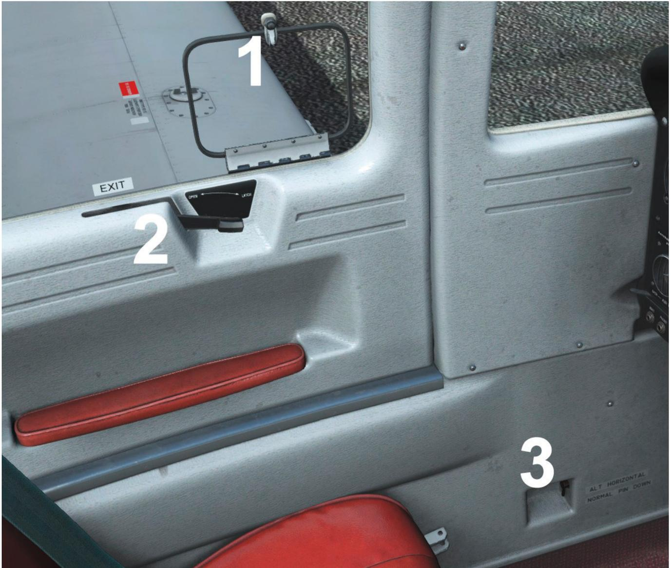
1. Storm window (note that the latch must be moved prior to opening/closing the window)
