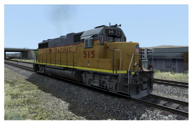
The GP38-2 is an upgraded version of General Motors GP38, differing in only minor details. Its 16-cylinder engine generates 2,000 horse power and the class remain in service to this day due to their reliability and ease of maintenance.
